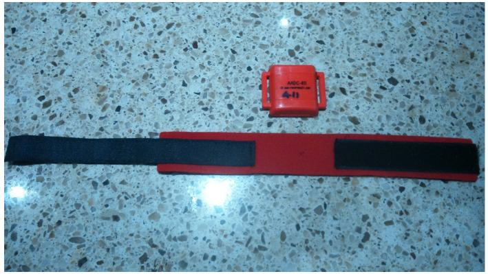
Now peel the velcro away from the neoprene and thread the velcro up and over the tag through the loops on the tag as shown:
